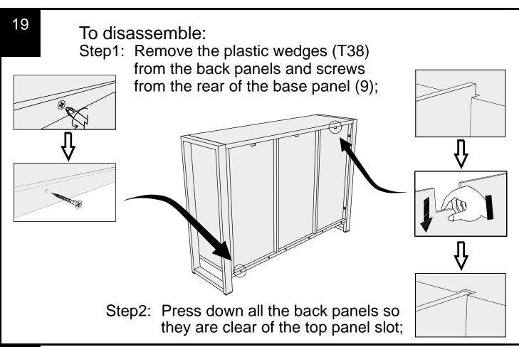
Slide the top panel front to unlock, then lift off. Follow the same sequence to remove the other panels;
