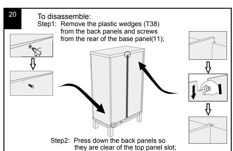
21 Slide the top panel front to unlock, then lift off. Follow the same sequence to remove the other panels;
