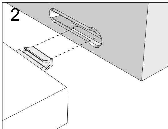
Push connector into housing to join.
