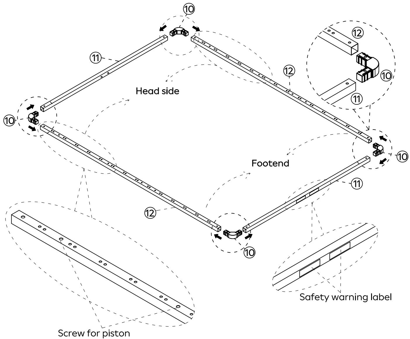
Note: The tube ⑪ with safety warning label should be assembled footend.
