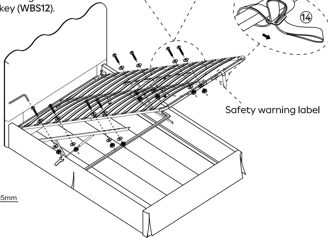
We suggest to assemble the slat frame in the middle position of the bed and try to keep 15mm distance on both side rails and keep 12mm distance on headboard and footboard, need to be equidistant.
