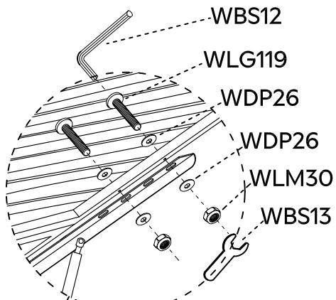
Fix the nut (WLM30) at one end of bolt (WLG119) by using spanner (WBS13), then tighten the bolt (WLG119) by using allen key (WBS12).
