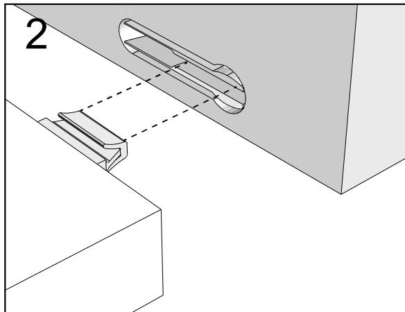
Push connector into housing to join.
